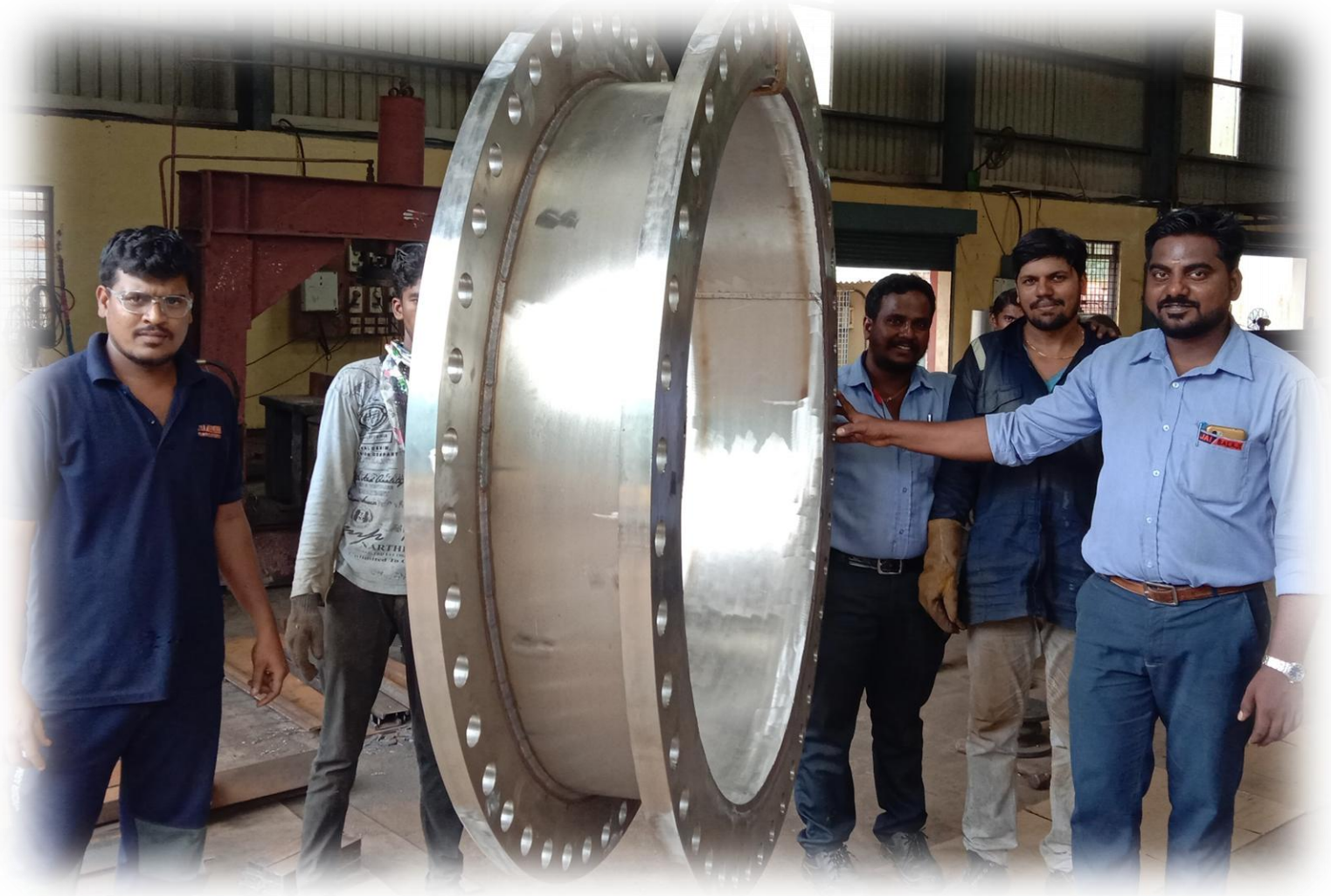
Spool – SS316L 50mmthk Flange, 20mm Shell
